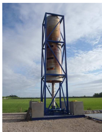
B – single tip shrouded flare
